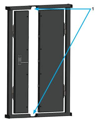
1. Wood blocks at top and bottom to protect the frame from explosive charge and cutting.
